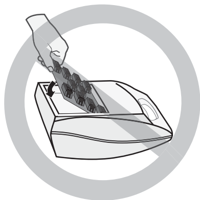
Figure 10: DO NOT install battery assembly this way.
