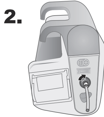
řekil 8-2 X Series Advanced nitesine Tek Lmenli Hortum Takma
